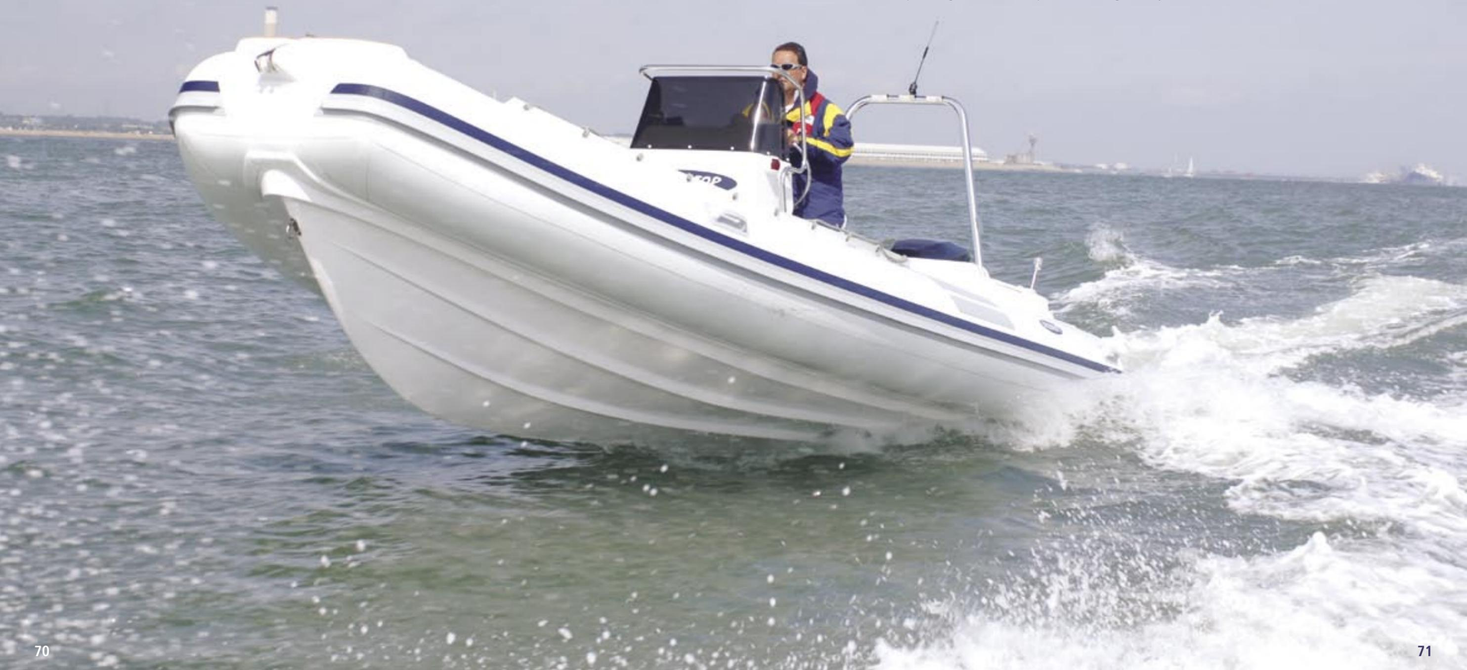
►►A further benefit of this squared bow concept is to reduce overall length without reducing hull length, and it makes it easier for boarding over the bow. In the bow, steps have been moulded on the top of the stem and as a locker lid for the rope locker. It all fits very sweetly.
