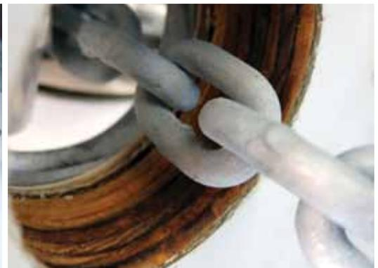
The unprotected plywood edge below the windlass needs protecting.
