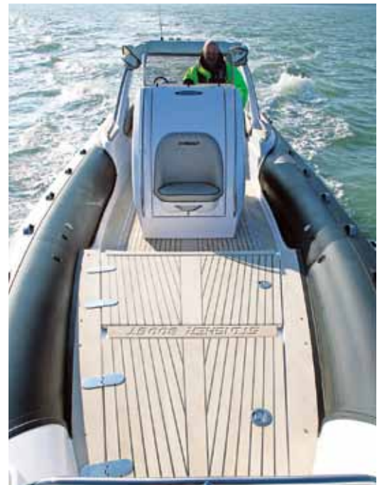
The long foredeck now has a machined insignia cut into the Flexiteek
