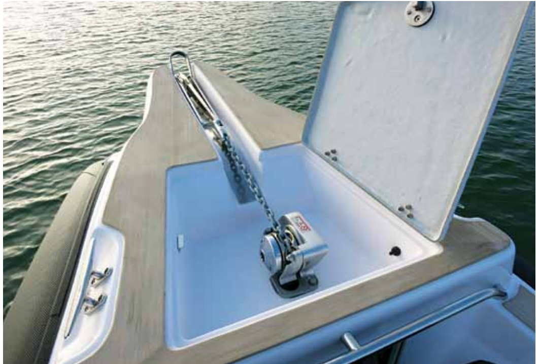
The grab handle behind the anchor locker proves remarkably useful underway
